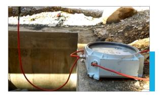
The researchers of UT managed to employ a method to measure electrochemical noise and monitor and control corrosion of oil and gas pipelines for the first time in the country. In this method, noise is measured through analysis of
